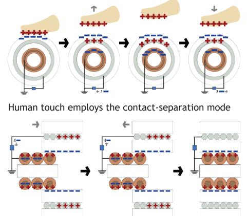
Force along the axis (e.g., stretching) of the cord induces a lateral sliding mode TENG
