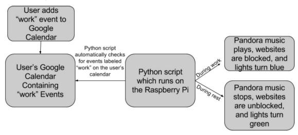
Our prototype has been designed to be a context aware, interface-less device with a very minimal setup requirement for the end user. On the device, a Python script runs at startup to automatically check the user's Google calendar and activate the device during work times. In its current iteration state, the prototype user only needs to interact with prototype to customize default settings in the three following parts:
