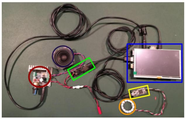
From left to right, our hardware components are as follows: 12-volt external audio amplifier (circled in red), 2.5" speaker (circled in purple), 12 volts to 5v USB buck convertor (green rectangle), 12 LED NeoPixel ring (circled in orange), Teensy 3.2 microcontroller (yellow rectangle), Raspberry Pi Model 3 (shown here with a 5" TFT touchscreen used for debugging, in blue rectangle).
